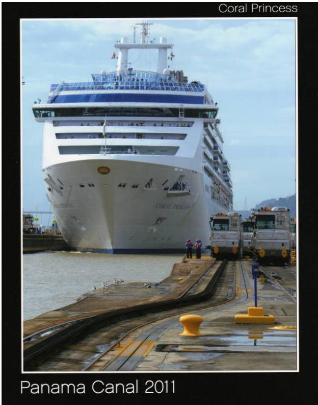
The mules run on rack tracks to which they are geared. Each mule is equipped with a winch which is operated by the driver who either pays out or takes in the line attached to the ship this is to hold her central in the lock whilst moving from chamber to chamber. With a ship the size of Coral Princess this takes considerable skill as the lock chamber is only 4 ft wider than the ship! (See picture 1)
