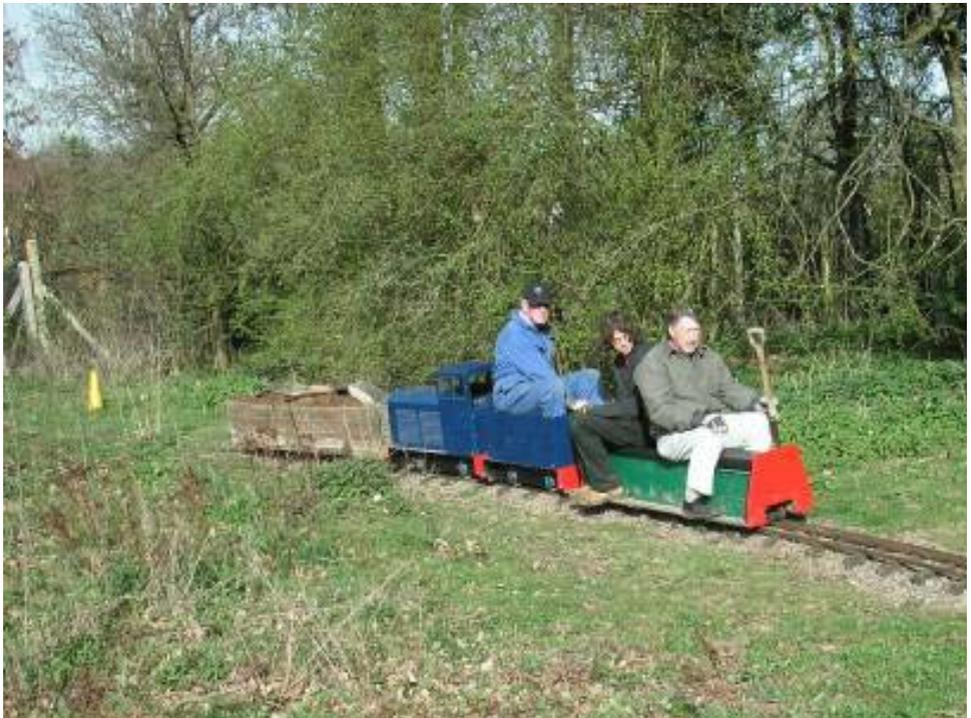
Roys engineers train bringing a wagon load of spoil from the car park to make the new embankment. Photo: Geoff Burton
